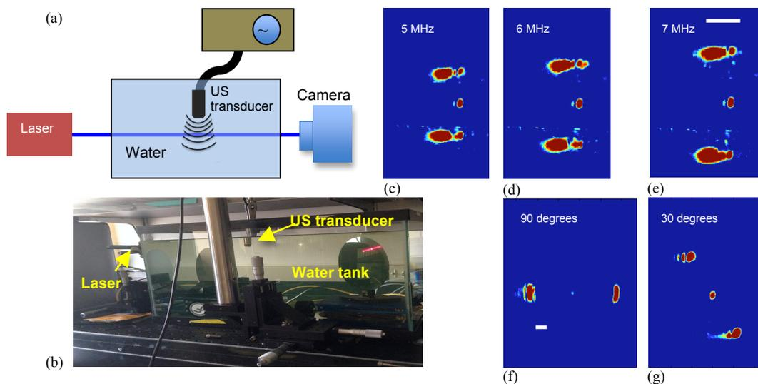
Fig. 2 (a) Schematic of the characterization setup. (b)-(d) Normalized light intensity patterns demonstrating that by changing the location of two diffracted beam patterns, we can scan a biological tissue. (e) and (f) show the effect of the angle change to steer the optical beam pattern. Scale bars are 2 mm. (c)-(e) share the same scale bar. (f)-(g) have the same scale.
