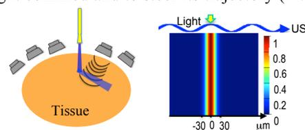
Fig. 1 (a) Schematic of optical beam steering in a tissue using ultrasonic waves. (b) FEM simulation showing the possibility of optical light waveguiding in high-pressure zone of a propagating US wave at  $15\text{MHz}$ .
